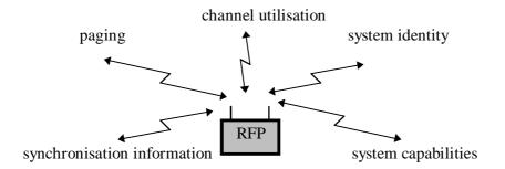
Figure 5. The DECT fixed part beacon function
