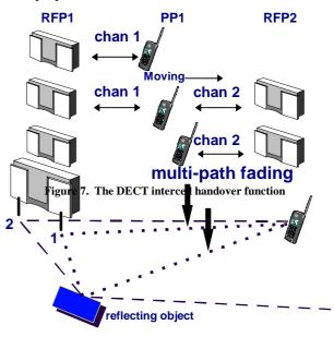
Figure 8. Antenna diversity from 1 to 2
